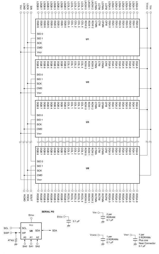
Remarks 1. Rambus Channel signals form a loop through the RIMM module, with the exception of the SIO chain.
